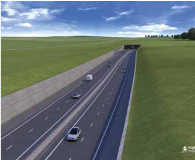
Fig. 4: Proposed approach to west tunnel portals. Note the lacking indication of heavy traffic, signage and lighting.
