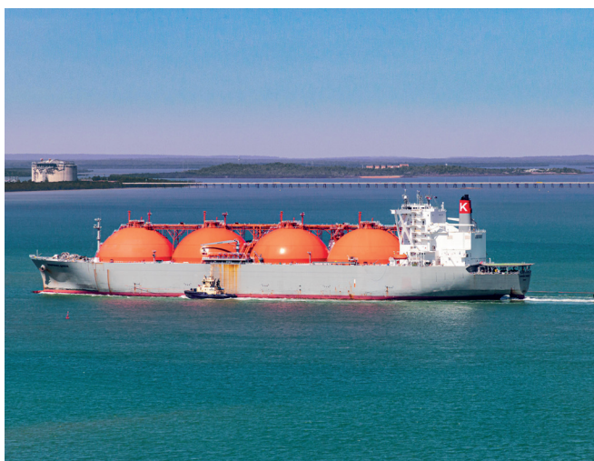
Fig. 3: A typical LNG tanker. Standard vessels of this kind are often over 270 m long and around 45 m wide, while the largest can reach up to 345 m in length and 55 m in width, highlighting the massive scale of maritime traffic associated with LNG export terminals.
